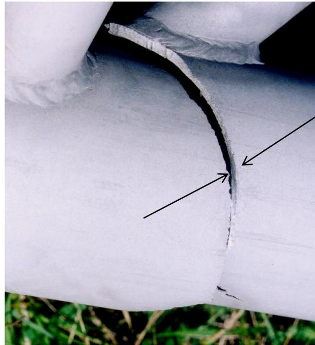
The crack propagated circumferentially around the chord member until complete separation.
