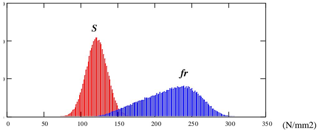
Figure-13 Histogram of acting stress  $S$  and deteriorated strength  $fr$
