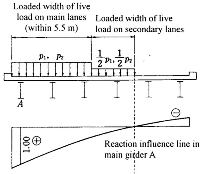
Figure-5 Transverse Reduction of L-Load (SHB)
