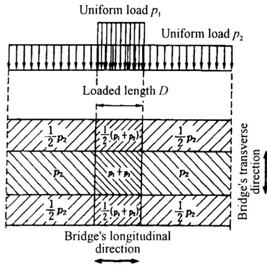
Figure-8 Loading Pattern of L load (SHB)
