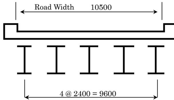
Figure-7 Cross section of the object Bridge
