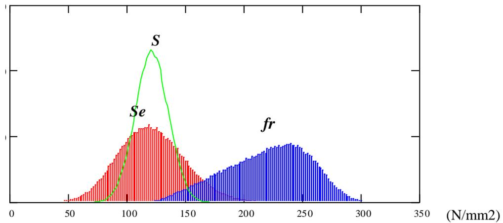
Figure-14 Calculated Histogram of Diffused acting stress  $Se$  and deteriorated strength  $fr$
