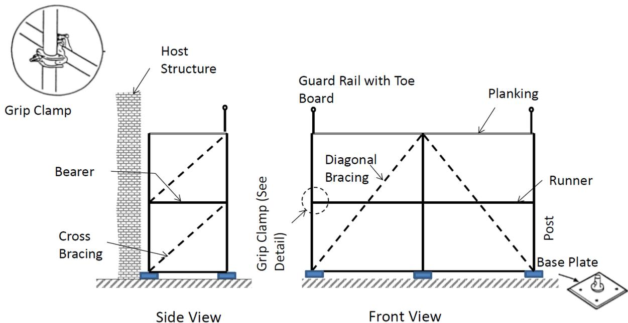
Figure 1. Schematics of a tube and coupler scaffold
