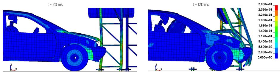
Figure 7.: von-Mises stress ( $v_{init} = 50$  km/h) at  $t = 120$  ms
