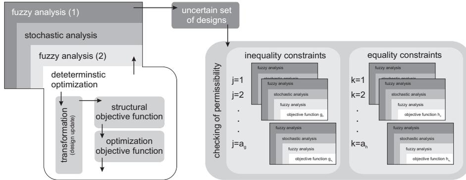
Figure 5.: Framework for computing the optimization task with the passive approach
