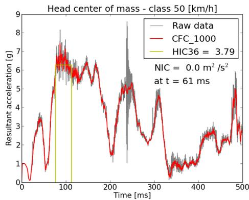
Figure 8.: Acceleration time dependency of the head
